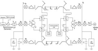
Figure: 1 Basic model for composite ac-dc transmission.
