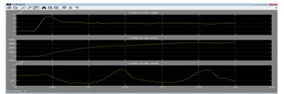
Fig 9: Rectifier DC side (voltage, Current), Inverter dc side voltage
