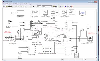
Fig 4: Simulink Model (Double line circuit) using Simultaneous AC-DC Transmission
